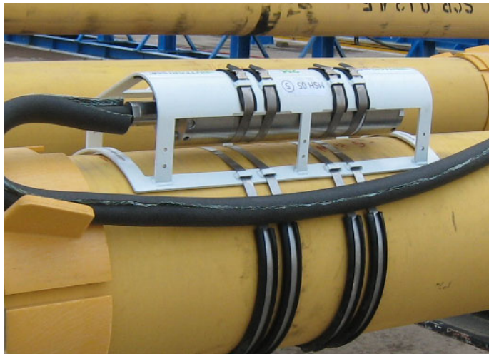
Figure 2 –INTEGRIPod Motion Sensor Installed on SCR Joint
