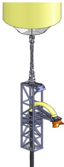
Figure 4 – Jumper Offtake below Buoyancy Tank
