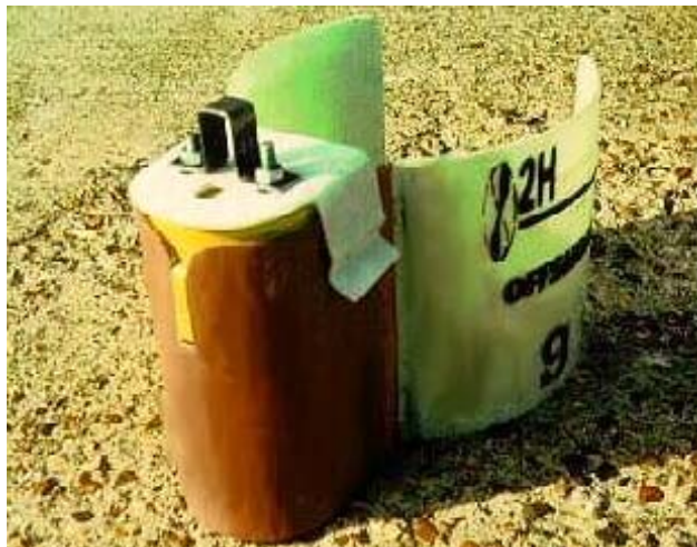
Figure 2 – Logger Bottle within Riser Attachment Assembly
