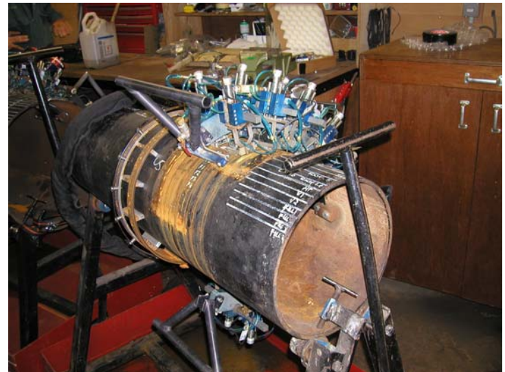
Figure 7 – Calibrating Automated Ultrasonic Testing (AUT) System
