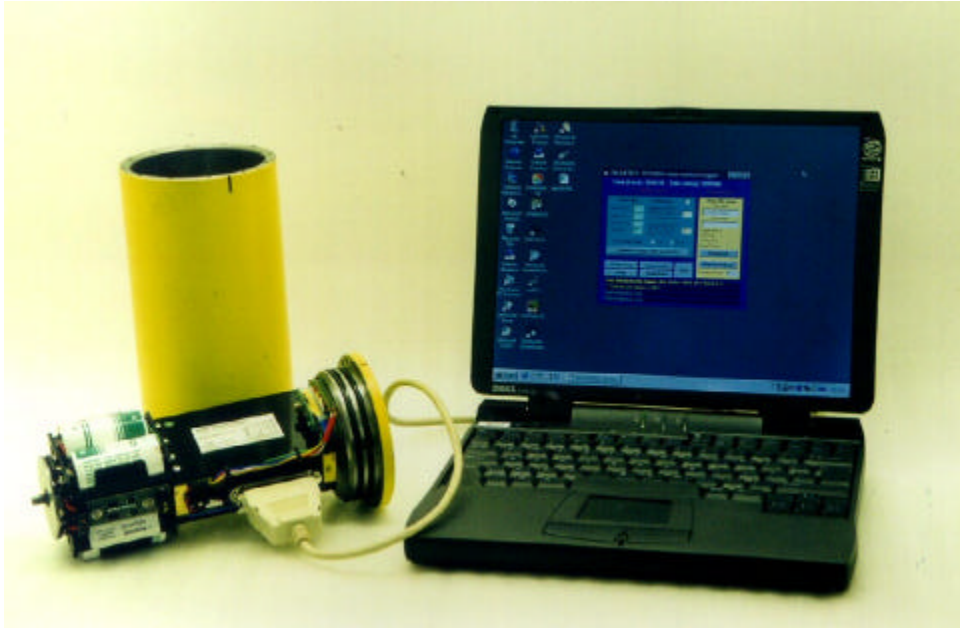
Figure 2 - 2H Accelerometer Data Logger
