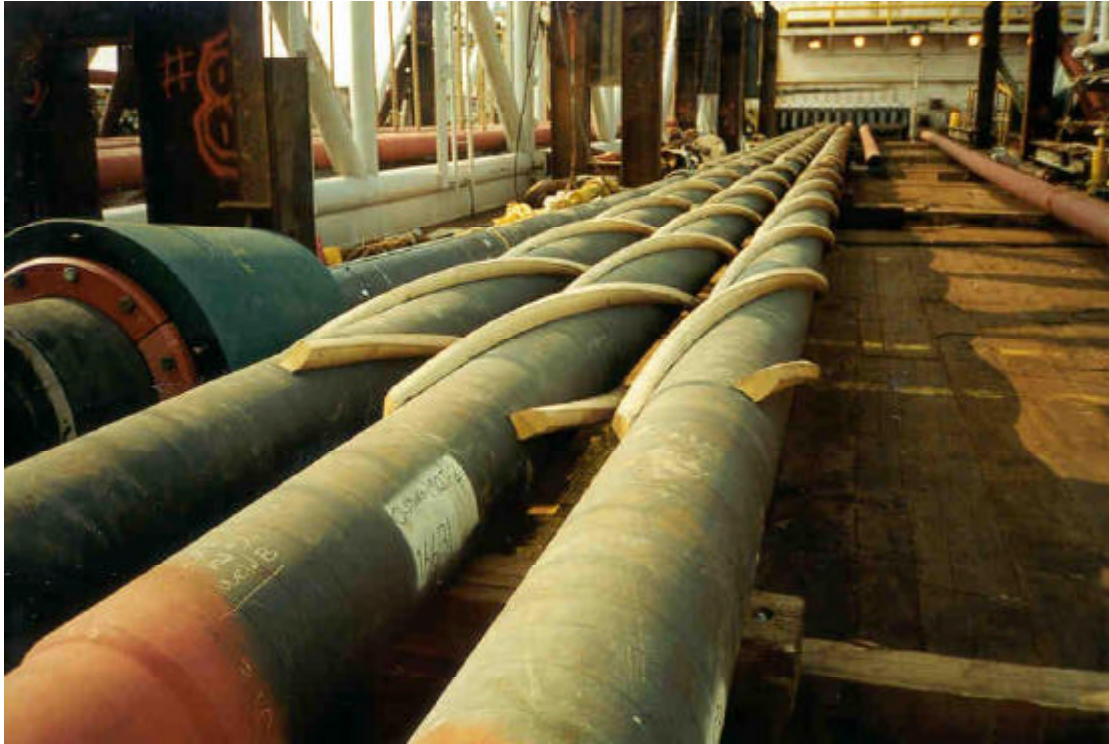
Figure 3 – Helical VIV Suppression Strakes
