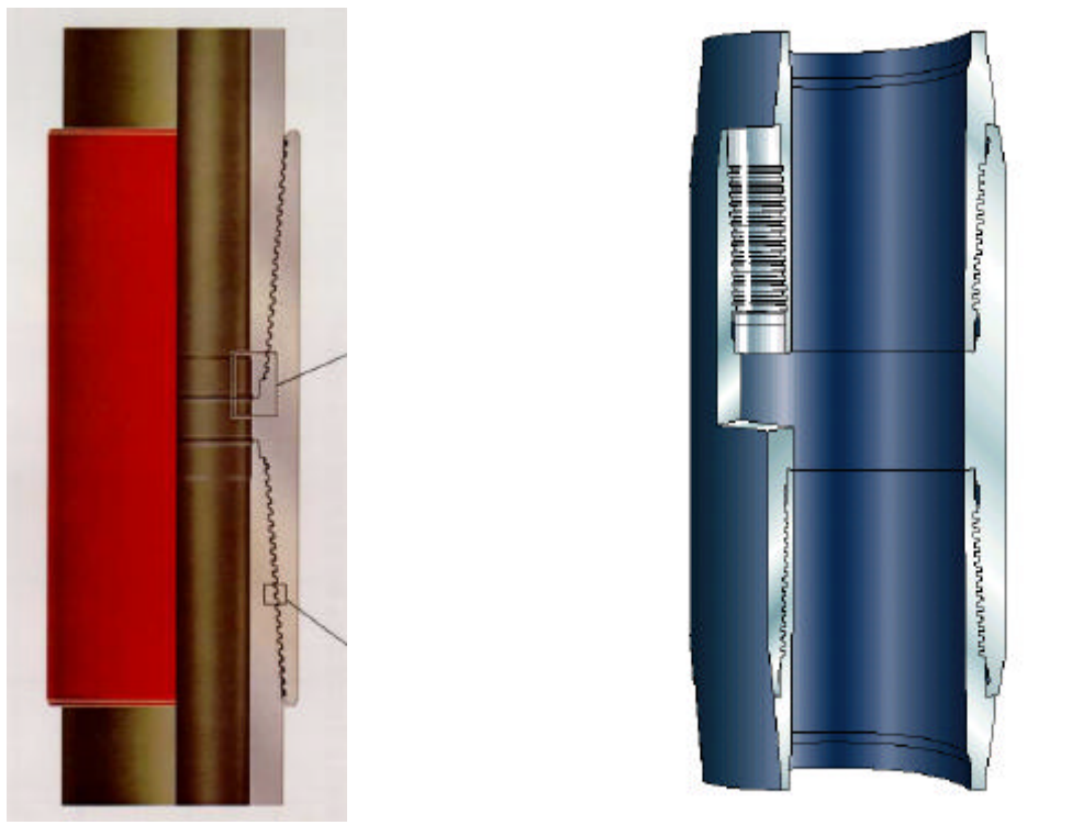
Figure 3 - Standard Casing Connector and Modified Casing Connection
