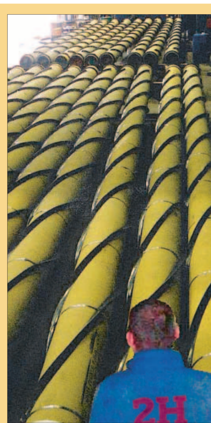
Above and right: all riser types must guard against VIV Photos: 2H OFFSHORE
