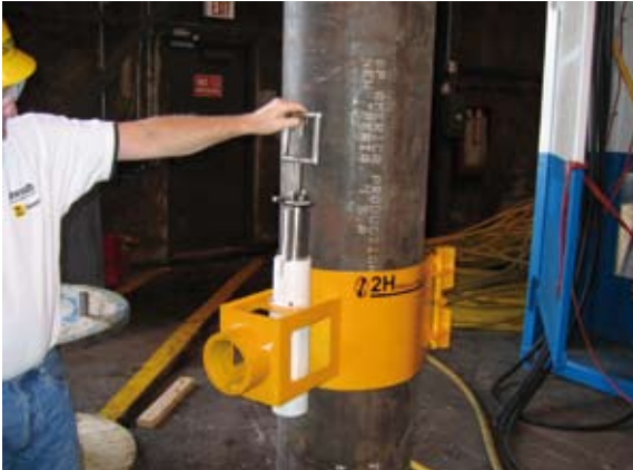
Above: Deploying riser monitoring systems Top row: Curvature sensors (developed by Insensys) using optical fibres are attached to a riser to determine the shape and bending stresses along its length Bottom row: Accelerometer bottles (from 2H Offshore Engineering) are deployed for riser data logging on several BP platforms in the Gulf of Mexico, and on drilling risers (circled in white)
