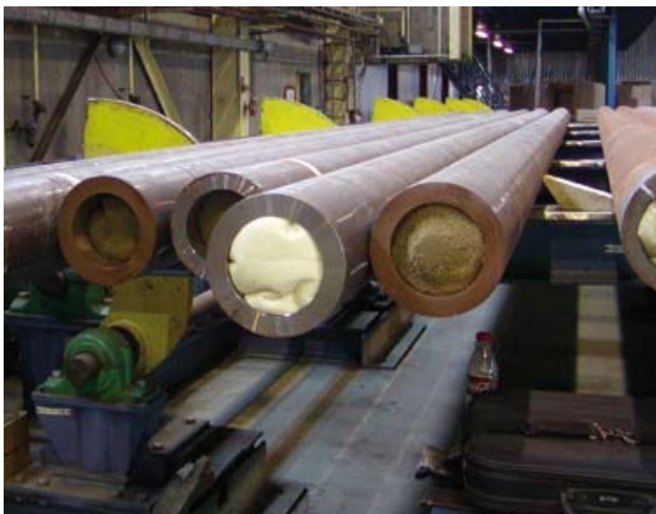
Joints of pipe used to construct a deepwater riser. In this case the pipes are 160mm internal diameter, with wall thickness of 40mm
