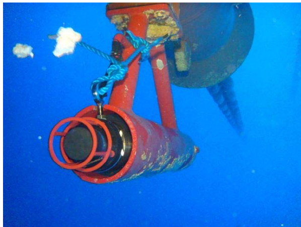
Figure 11 – Right: Diver/ROV Replaceable INTEGRipod Connected to Chain Follower in Shell BC-10, Espirito Santo FPSO.
