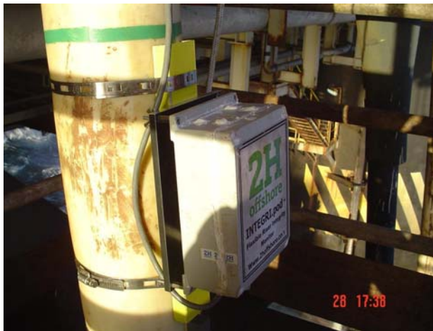
Figure 16 – Left: View of flexASSURE Sensor in a Prototype Casing Installed Offshore. Figure 17 – Right: Artistic Schematic View of Sensors Installed Subsea.
