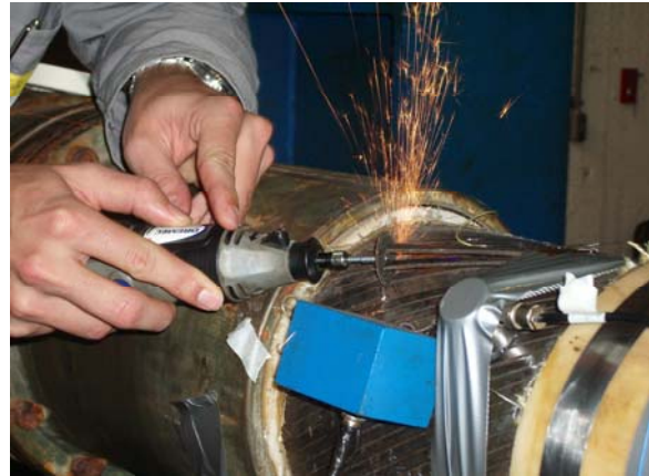
Figure 14 – Left: flexASSURE Lab Test at COPPE, Federal University of Rio de Janeiro, Brazil. Figure 15 – Right: Notch creation on Armour Wires During Lab Test.
