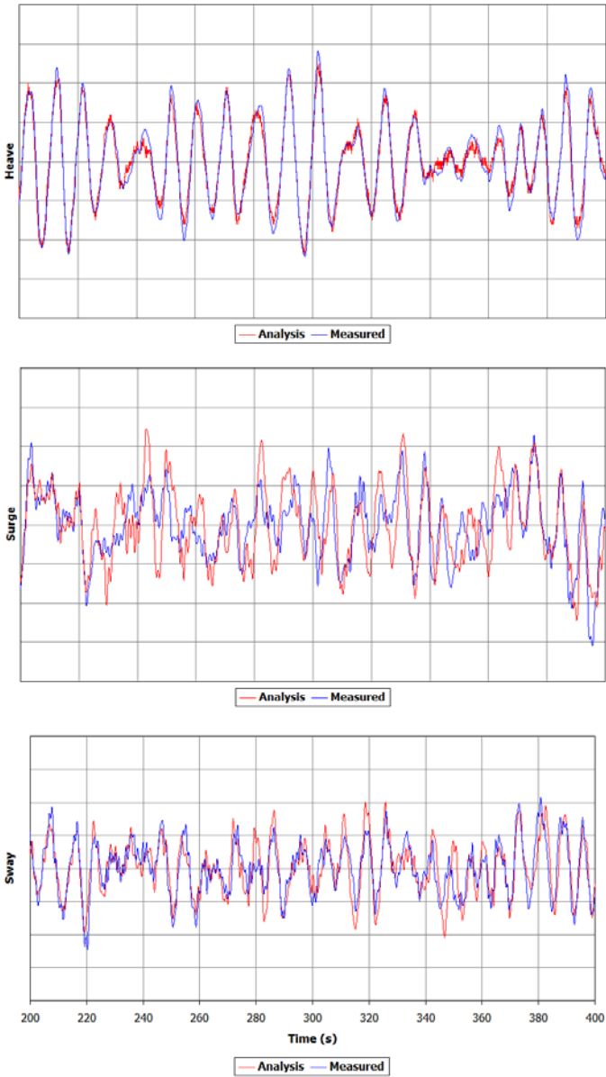
Figure 3: Riser acceleration comparison of measurements against analysis predictions at hang-off device 3 location.
